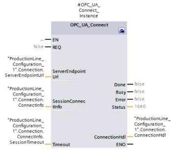
"ProductionLine" is the interface that the OPC UA client of the example (Page 308) uses for data exchange with the OPC UA server "ProductionLine".
