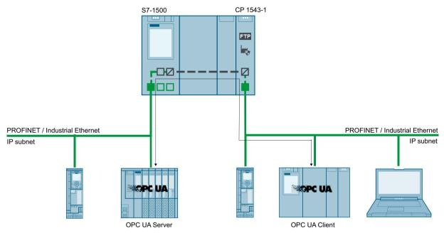
Figure 10-3 Example: Access of OPC UA clients to OPC UA servers via S7-1500 CPU with activated IP Forwarding
