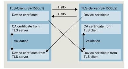
Figure 4-24 Certificate handling for Secure OUC between two S7-1500 CPUs
