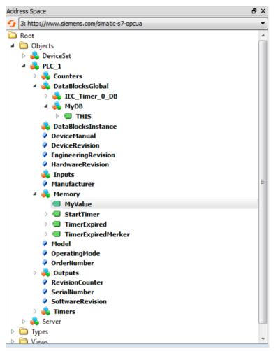
Figure 10-8 Example of the address space of the OPC UA server of an S7-1500 CPU
