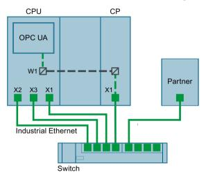
Figure 12-14 Principle of the virtual interface
