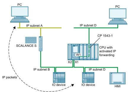
The following figure shows how to protect your automation system against unauthorized access.
