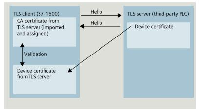
Figure 4-19 Certificate handling from the perspective of the S7-1500 as a TLS client
