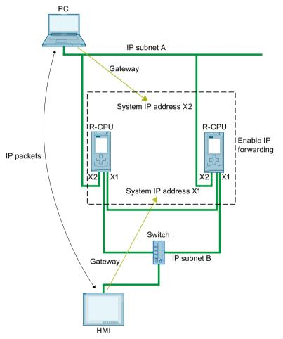
Figure 15-4 Example: IP forwarding via the system IP address
