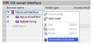
**Result**: STEP 7 generates the corresponding structure for the mapping in which you still need to adjust the required text length (Text) and the required locale (Locale) for "LocalizedText".
