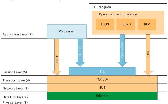
The figure below shows the TLS protocol in the context of communication layers.
