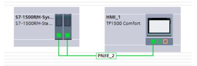
Figure 15-7 Networking an HMI device with the S7-1500R/H redundant system
