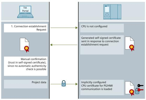
Figure 4-34 Connection establishment, provisioning phase
