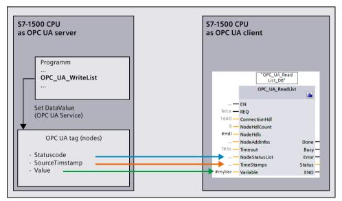
Figure 10-15 Client reads data value (OPC UA tag of the server of the S7-1500 CPU)
