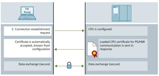
Figure 4-35 Startup of PG/HMI communication
