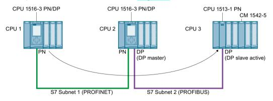
Figure 12-4 S7 routing via CPU-CPU communication
