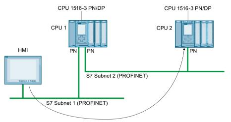
Figure 12-3 S7 routing via HMI connections
