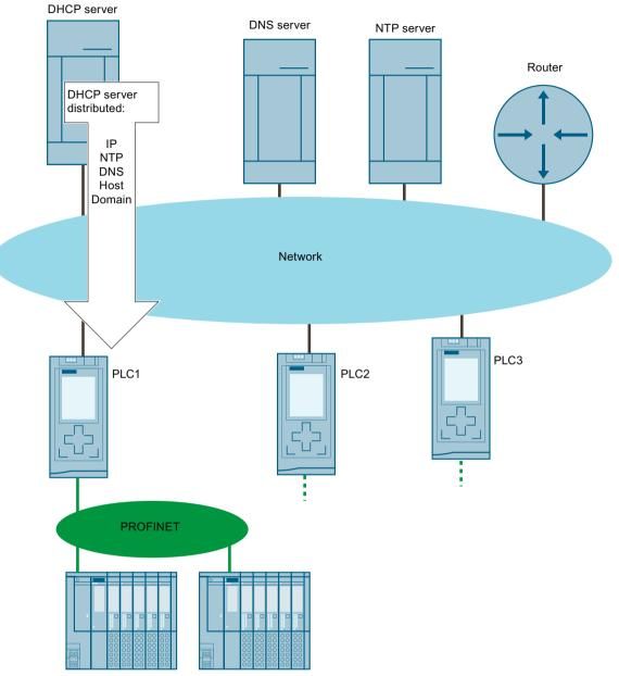
For the interfaces of an S7-1500 CPU you can set that address parameters such as the IP address with subnet mask, can be got from a DHCPv4 server (hereinafter DHCP server).
