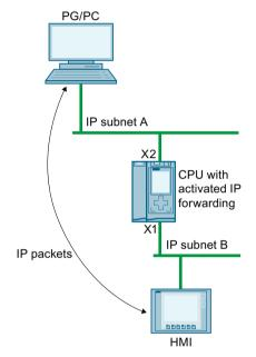
Figure 12-6 Access of a programming device to an HMI via IP forwarding
