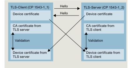
Figure 4-28 Certificate handling in secure OUC between two S7-1500 CPUs via CP interfaces.
