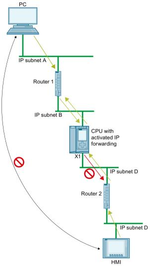
Figure 12-9 Unsupported IP router cascade
