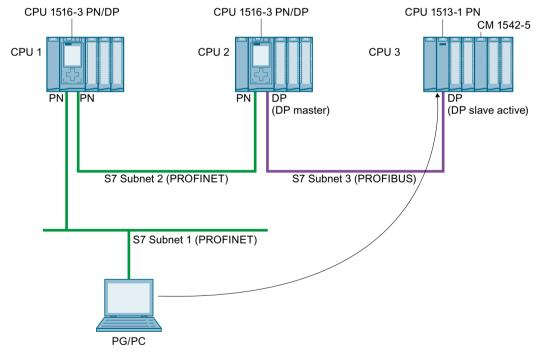
Figure 12-2 S7 routing: PROFINET - PROFIBUS
