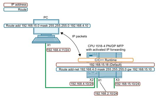
Figure 12-10 Access to C/C++ Runtime via interface X2
