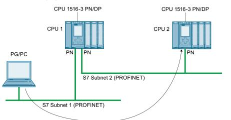
In the following figure, CPU 1 is the S7 router between S7 subnet 1 and S7 subnet 2.
