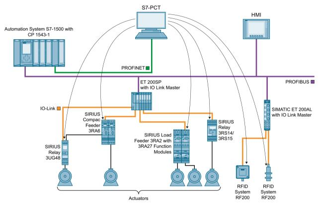
The figure below shows an example configuration with the data record routing with PCT.
