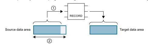
① The source data area is smaller than the maximum size of the consistent data area (②). The instruction transfers the data together to the destination data area.
