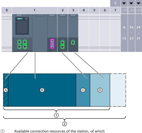
The figure below shows an example of how individual components make connection resources available to an S7-1500 station.
