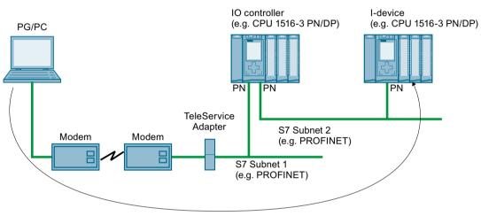
Figure 12-5 Remote maintenance of a plant using TeleService
