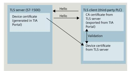
Figure 4-22 Certificate handling from the perspective of the S7-1500 as TLS server
