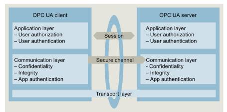
Figure 10-6 Necessary layers: transport layer, secure channel and session
