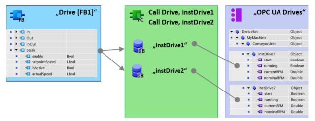
By mapping between FB type information / UDT type information and OPC UA type information, STEP 7 is able to create all instances present in the program as nodes in the server interface.
